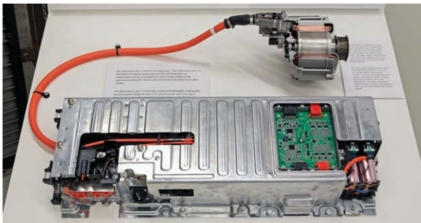
Figure 8 Buick's eAssist comprises a 0.5-kWhr, 32-cell battery pack, control electronics, and a 15-hp motor/generator to augment the four-cylinder engine on a Buick LaCrosse, making it a light hybrid. This display of components shows a shorter cable to save space. In the vehicle, it runs from the battery over the rear axle to the motor/generator mounted on the engine.
