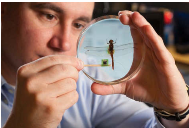
Researchers at Duke University have developed a wirelessly powered, lightweight, and powerful telemetry system that allows scientists to study the neurological activity of dragonflies as they capture prey. You can just barely see the threadlike antenna end hanging down on the right.
