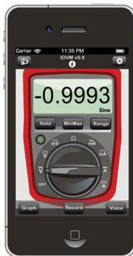
Figure 4 A wireless digital multimeter from Redfish Instruments lets you remotely view and log measurements over a Wi-Fi network.
